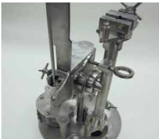
Fig. 4.12. Equipment to open round vials with irradiated cobalt
